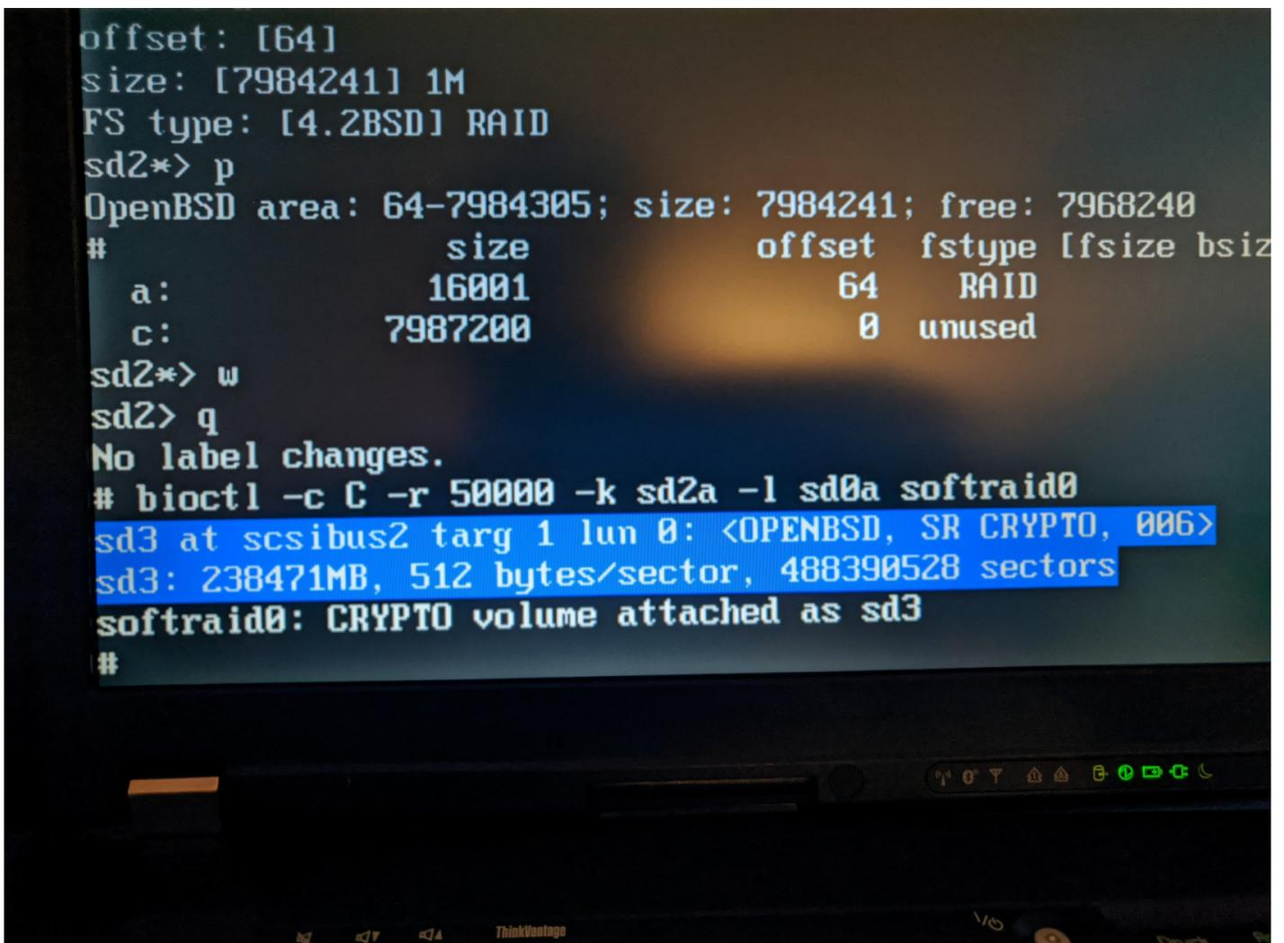
A terminal window screenshot showing the execution of bioctl and the resulting output. The terminal output is as follows:
